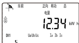
Current forward active energy 12.34kWh
