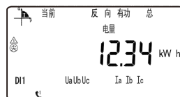
Current reversing active energy 12.34kWh
