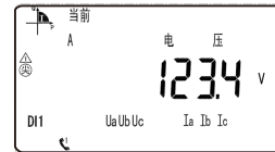
Voltage on A phase is 123.4V
