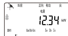
Current forward active energy 12.34kWh
